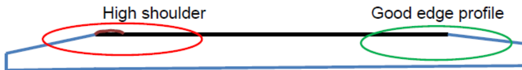
FIG. 1 – Gypsum Board Cross Sectional View
